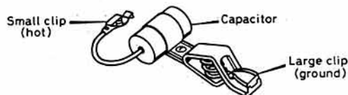
Fig 8. Use of a capacitor "touched" in turn to "hot" electrical points in order to trace sources of interference
